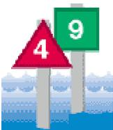
**Daymarks** are permanently placed signs attached to structures such as posts in the water. Common daymarks are red triangles (equivalent to nuns) and green squares (equivalent to cans) and may also be lighted.
